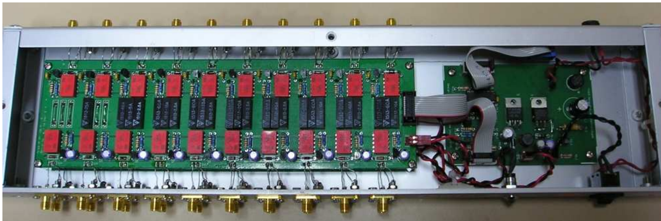
Figure 1: The inside of the HAARP phasing box showing the solid state delay lines (black) for ten of the antennae with the logic circuit on the right
