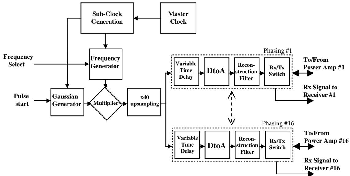
Figure 4, Proposed TIGER Digital Transmitter - Block Diagram
