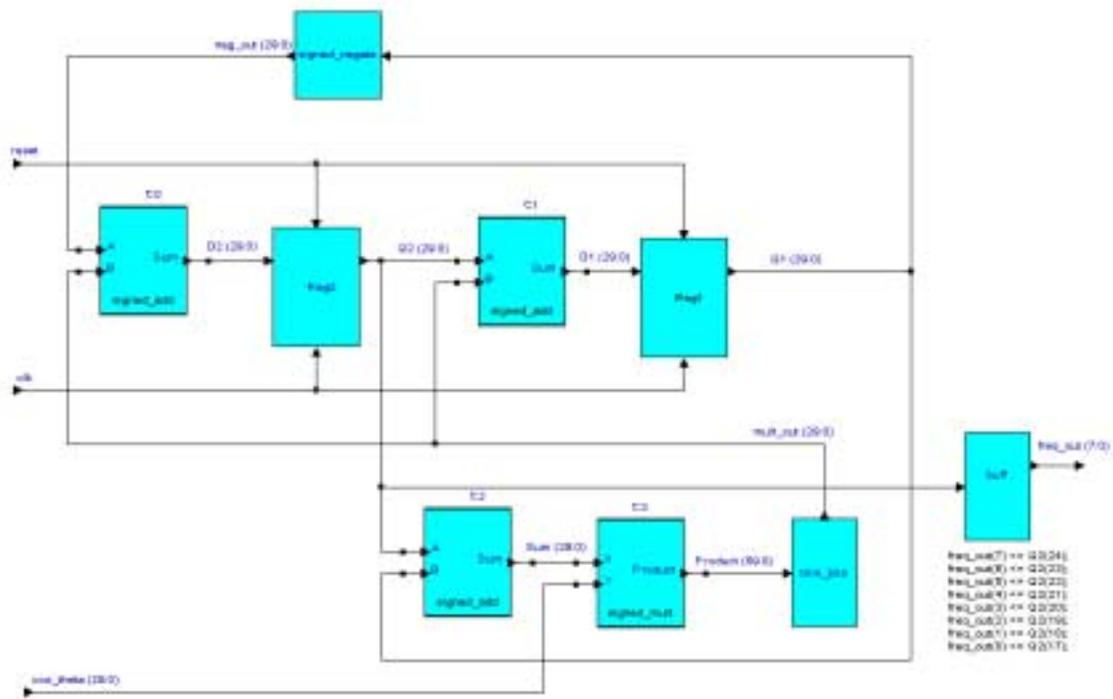
Figure 9, Frequency Generator - Block Diagram
