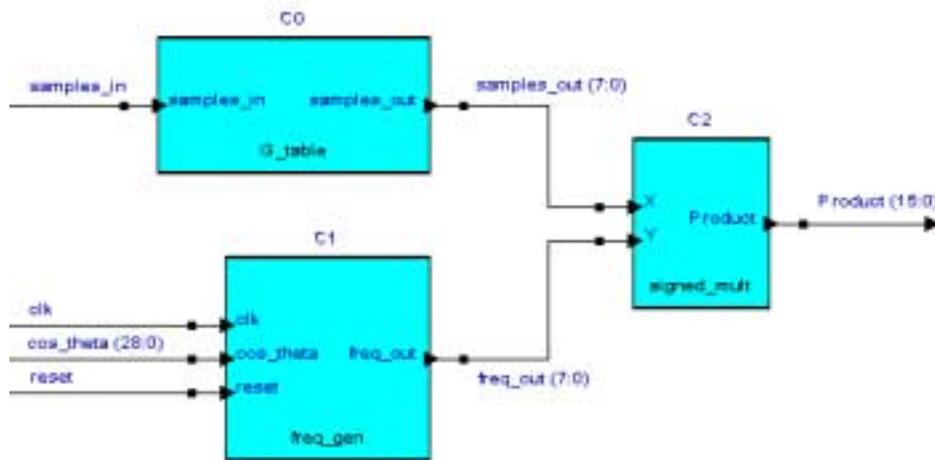
Figure 5, Gaussian Pulse Modulator - Block Diagram
