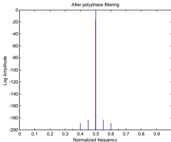
Figure 12, Polyphase Filer Normalised Frequency Response
