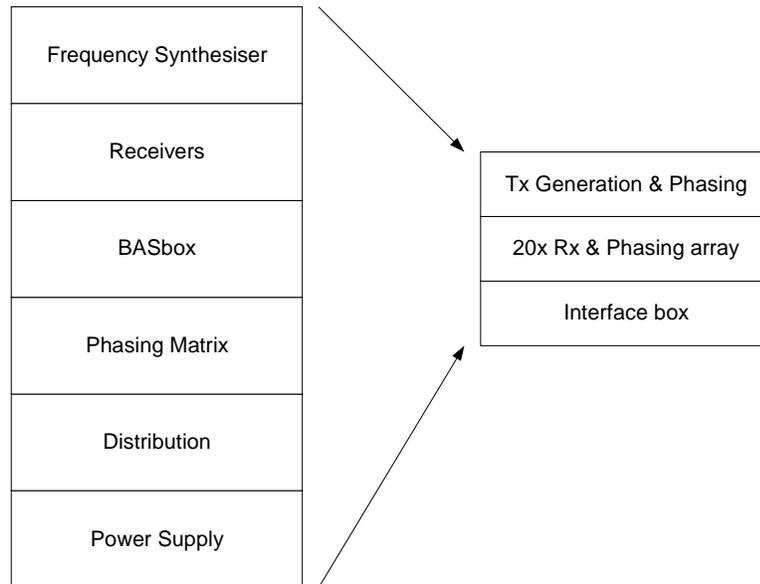
Figure 3, Proposed Reduction of Left Hand Rack
