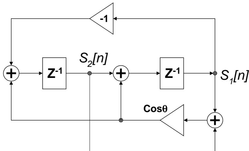
Figure 6, Single Multiplier Sine-Cosine Generator
