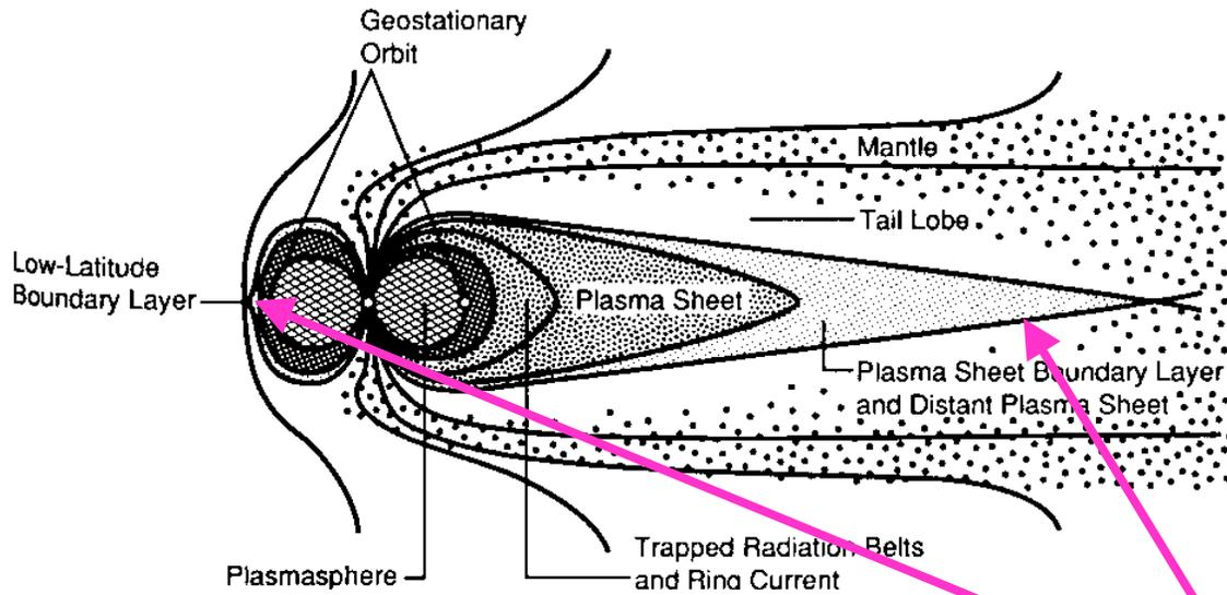
**FIG. 10.4.** Schematic diagram of plasma regions of the earth's magnetosphere as viewed in the noon-midnight meridian plane. The plasmasphere typically occupies much of the same region of space as the radiation belts. Frequently there is little or no gap between the inner edge of the plasma sheet and the outer boundary of the trapped radiation belts.
