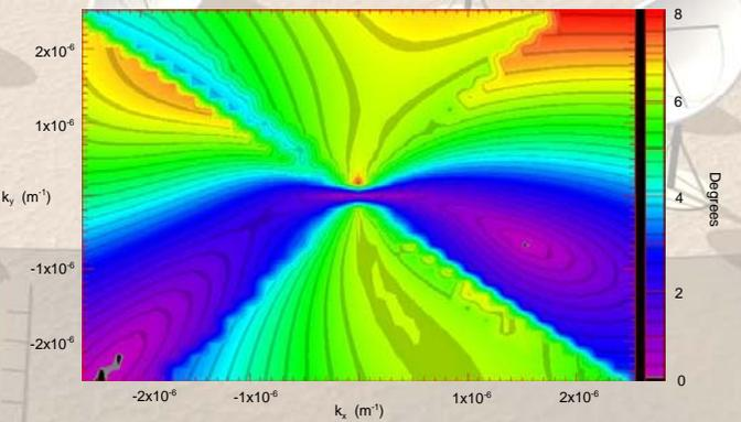
Figure 4: Phase delays (in Degrees) for a 70MHz signal affected by a 65mHz ULF wave with 5 nT (horizontal component perturbation) at the ground.
