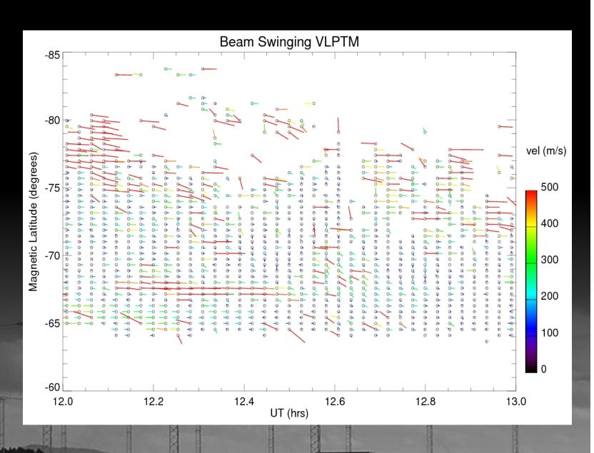
Beam swinging shows an Auroral Eastward Flow Channel from 1206UT to 1236UT in the premidnight sector at 68° Latitude
