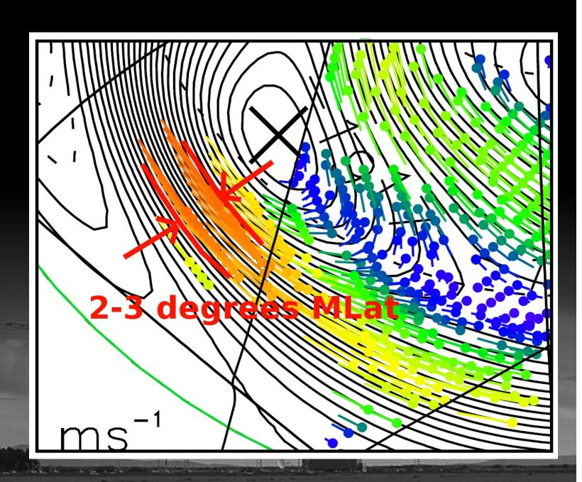
Between 1206UT and 1236UT an Auroral Eastward Flow Channel manifests on the poleward edge of the Harang "Banana" within the TIGER radar field of view
