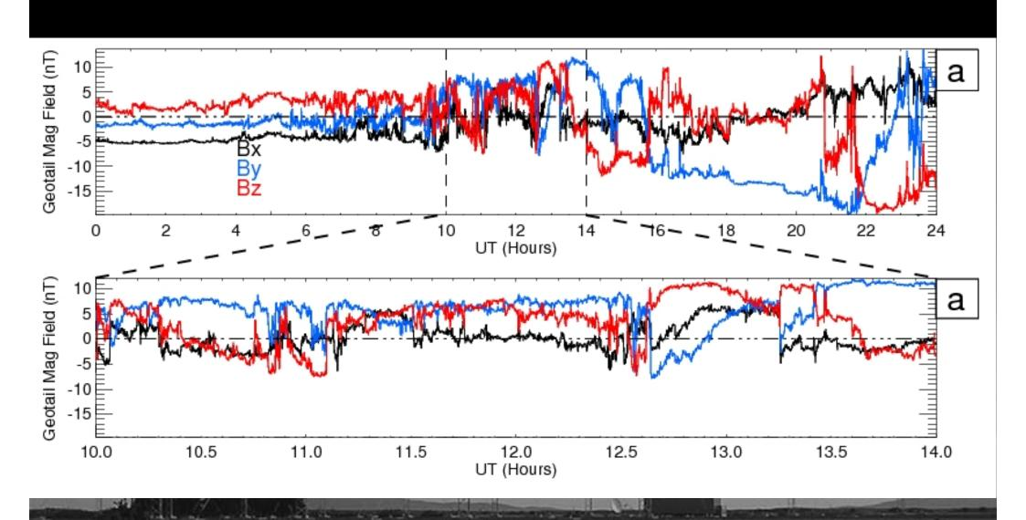
Two intervals, 1015 – 1106UT and 1226 – 1238UT, where the IMF component Bz is negative (red curve) and By is positive (blue curve)
