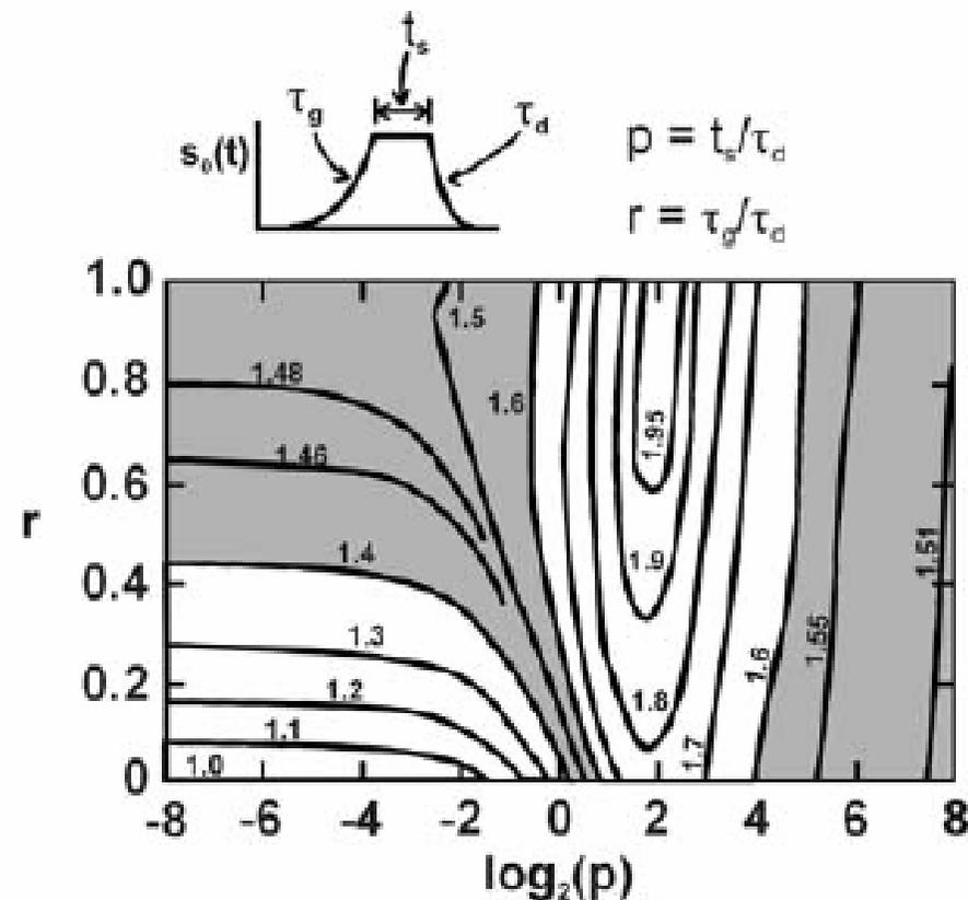
Figure 2. Values of  $n_\tau$  obtained by fitting with an exponential power law (equation (2)) the ACF magnitude (equations (13) and (14)) of the scatterer model (equation (12)) shown at the top of the figure. The curves are contours of constant  $n_\tau$ .
