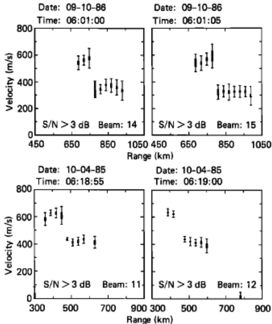
Fig. 7. Example of transition between both kinds of high Doppler velocities observed as looking along a single beam. The absolute value of the velocity is plotted as a function of range from the radar for the selected beam. Range gates are separated by 30 km. The conventions to plot the velocity with its error and the half-power are the same as for Figures 3, 4, and 6.
